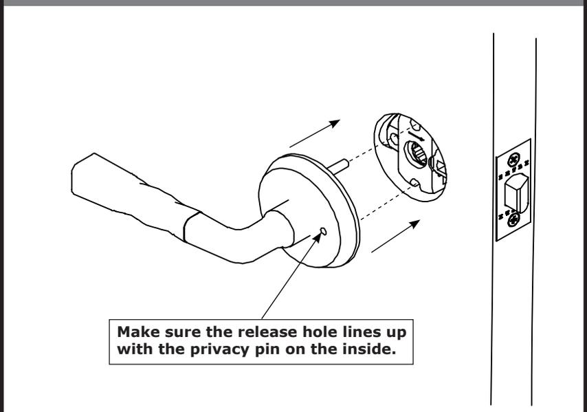
Step 2. Fasten Inside Trim using two #8 machine screws (provided), and install Privacy Pin.
