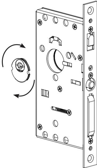
Note: Notches on cylinder must be parallel with the horizontal plane when fully screwed into lock body.
