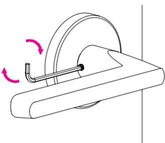
**Step 5:** Insert the short end of Allen wrench into the spindle and ensure that it is securely tightened.
