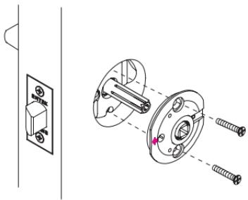
**⚠** Ensure the hole in the CF Mechanism aligns with the privacy pin hole in the Latch.
