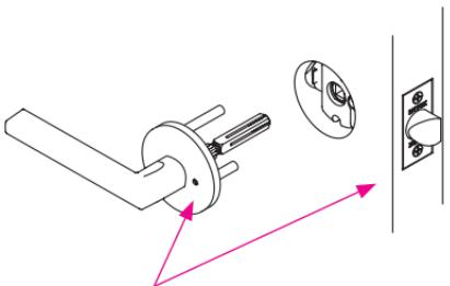
**⚠** If this handle set has a privacy function, ensure that the release hole is on the side closest to the edge of the door.
