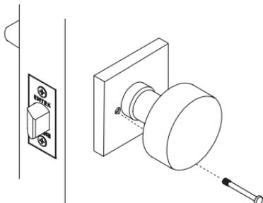
**⚠️** For emergency, insert a nail type object into the release hole of the exterior rosette to open the lock.
