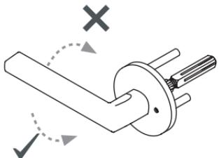
**Step 1:** Mount Pre-Assembled Trim, with the spindle entering the center of the plastic alignment tool.
