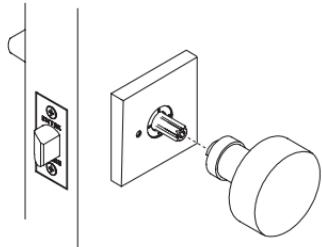
**Step 5:** Firmly tighten the Pre-installed set screw in the lever or knob with the provided Allen wrench. Ensure that it is firmly tightened.
