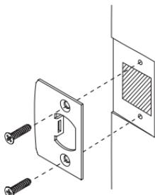
**Step 3:** Fasten Latch using two #8 x 3/4" wood screws.
