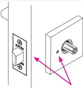
**⚠️** In the privacy function, ensure the privacy pin hole in the rosette is on the side closest to the door edge and aligns with the hole in the CF Mechanism.
