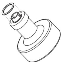
**Step 4:** Slide the door lever or knob onto the spindle. Make sure the plastic washer remains centered on the stem as you slide the lever or knob onto the spindle and up against the rosette.
