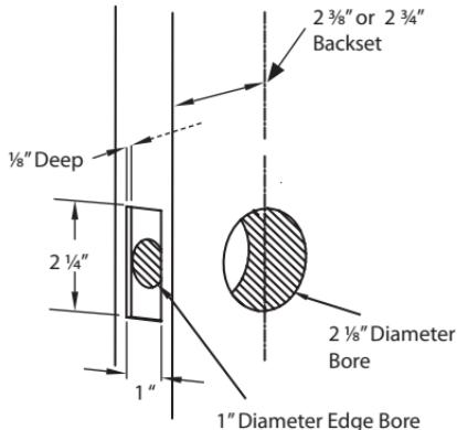
**Step 1:** Place Plastic Alignment tool in bore hole.
