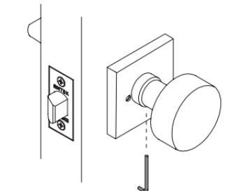
**Step 6:** For Privacy Lock, screw the Privacy Pin through the rosette, into the latch. To check functionality, turn the interior lever/knob to engage the latch. Now, push the privacy pin in and turn the exterior lever/knob. The exterior lever/knob should not retract the latch.
