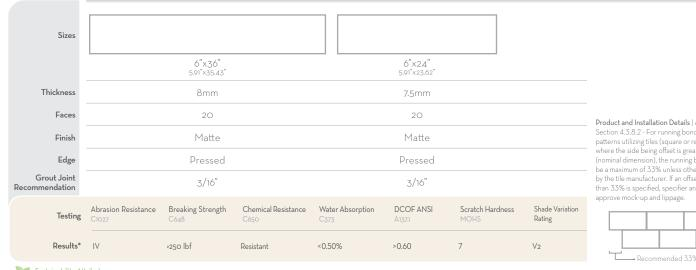
Product and Installation Details | ANSI A108.02 Section 4.3.8.2 - For running bond/brick joing patterns utilizing tiles (square or rectangular) where the side being offset is greater than 18" (nominal dimension), the running bond offset will be a maximum of 33% unless otherwise specified where the normal production of the second by the tile manufacturer. If an offset greater than 33% is specified, specifier and owner must approve mock-up and lippage.
