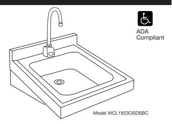
supply line. Control circuit is solid state, has adjustable sensor range (6" [152mm] preset to 30" [762mm]), shut off delay preset at 1 second and field adjustable to 2, 4 or 8 seconds, and automatic time-out feature (to prevent sink overflow) is preset at 0 seconds and is field adjustable to 15, 30 or 60 seconds.
