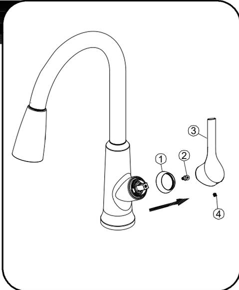
Shut off water supply. Unscrew the set screw (4) on the handle (3). Remove the handle (3) and loosen the screw (2) from valve stem. Loosen the cap (1).
