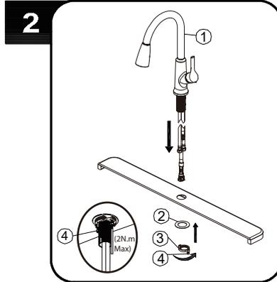
Place faucet (1) through the hole in the countertop. Secure the faucet (1) to the countertop using the metal washer (2), and mounting nut (3) provided. Tighten screws (4) with a phillips screwdriver. Do not overtighten.
