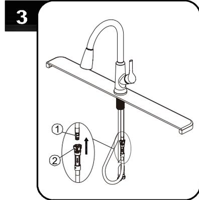
Push the quick connector (2) firmly upward and attach it to the receiving block (1). Pull down moderately to ensure the connection has been made.
