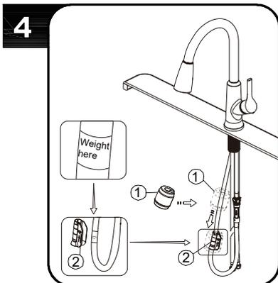
Install the weight clip (2) at the point of the hose marking "Weight here". Insert the weight (1) onto the clip (2) by sliding it down onto the clip (2).
