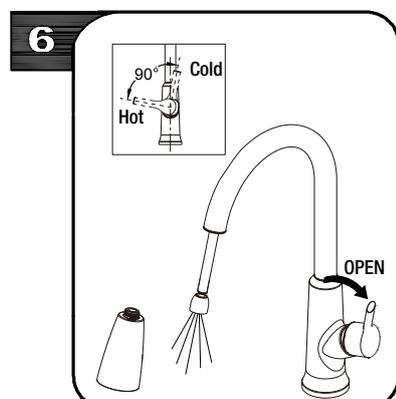
After the installation is complete, pull the hose assembly out of the spout and remove the spray head by unscrewing it from the hose in a counterclockwise direction. Turn on the water supply to flush debris from the faucet. Run the hot and cold water for at least one minute each. Important: This flushes away any debris that could cause damage to internal parts. Check for leaks.
