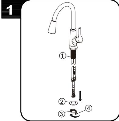
Before installation, shut off water supplies, remove old faucet. Next, remove metal washer (2), nut (3) and screws (4) from shank (1).
