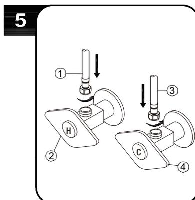
Thread the nut (1) on the hot water supply line onto the outlet of the hot water supply valve (2) and tighten with wrench. Do not overtighten. Thread the nut (3) on the cold water supply line onto the outlet of the cold water supply valve (4) and tighten with wrench. Do not overtighten.
