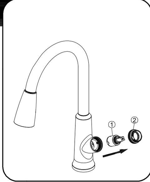
Loosen the cap (2) by turning it counter-clockwise and lift out the cartridge (1). Insert new cartridge. Reinstall the handle.
