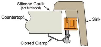
\*Maximum thickness for use of hold down system is 1-3/4" (44mm).
