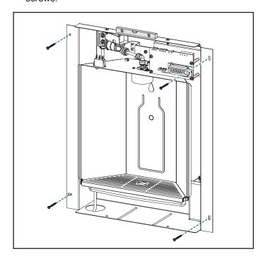
4. Locate the electrical gang box, at the lower right-hand corner of the water dispenser, and remove the cover.
