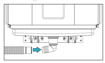
9. Route the drain hose through the filter box and attach the other end to the p-trap drain adapter using a hose clamp. The drain adapter is designed to be glued into a 1-1/4 inch PVC pipe.
