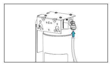
5. Connect the 1/4 inch water line to either a remote chiller or the 1/4 inch water line on the water dispenser. Use a union connection fitting to connect the water line to the water dispenser.
