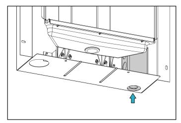
Note: If an optional filter unit will be installed under the water dispenser, the space behind that filter box is limited so make sure any electrical wiring will not interfere with mounting the filter box into the wall. Refer to "4.3 Critical Depth Dimensions" on page 6 for additional information.
