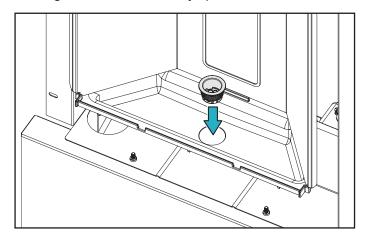
6. Install the O-ring over the strainer threads.
