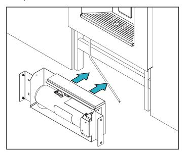
**Note:** Some side-to-side and up-and-down movement of the housing is capable to accurately align the filter unit with the water dispenser.
