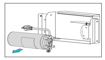
2. Securely mount the filter unit in the desired location.
