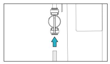
Connect a 1/4 inch water line, copper or plastic, to the outlet connector of the filter.
