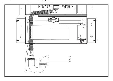
10. Connect the drain adapter into the household waste drain pipe.
