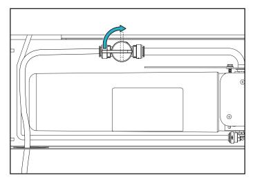
**Note:** The filter head contains an automatic shut-off valve that stops the flow of water, in case filter is inadvertently removed without shutting OFF the water supply.
