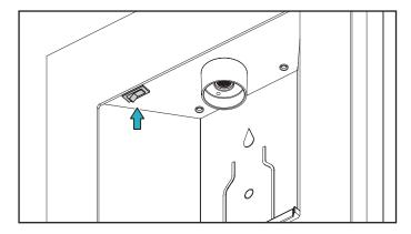
3. Move the power switch to the ON position and make sure the LED lights are lit.
