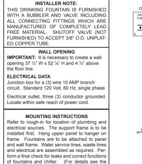
installation instructions.) Installation requires trap to be installed in wall. Trap and service stop not included.
