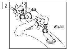
2. Use Teflon tapes on the threads of the mounting legs. Install the faucet body by connecting the end nuts of the water lines on the body to the mounting legs, Tighten the nuts.
