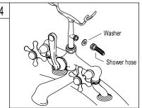
4. Place a washer between the side hole of the riser and the cone nut of the shower hose and tighten the cone nut.
