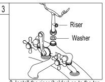
3. Install the riser (holder) on to the top connector hole of the faucet body. Tighten the end of the riser.
