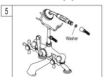
5. Place a washer between the hand held shower unit and the other end of the shower hose and then tighten the cone nut of the shower hose.
