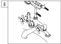
6. Turn on water supply and check for leaks. Allow both hot and cold water to run for one minute.
