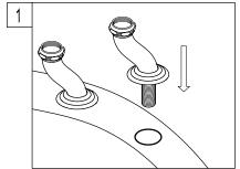
1. Place mounting legs on the tub, then tighten the lock nuts from underneath and connect the water supply lines. Place washers and then tighten the coupling nuts on to the mounting legs.
