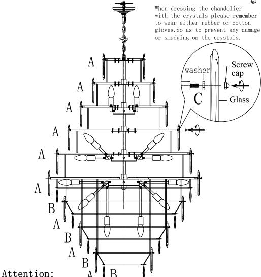
Install light bulb first before assembling crystal and glass. Please do not over-tighten!
