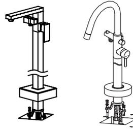
6. Insert the fixing bolts and fix tight in the floor. Move the cover to hide the base.
