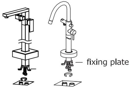
4. Insert the sliding cover on square pole, insert the flexible hose's snuts through the fixing base and connect the G 1/2 nuts with the water net connectors fixing tight by key.
