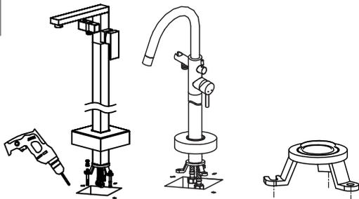
5. Adjust the complete to get correct position, then drill to fix base plate.
