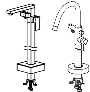
2. Match the square pole with the main body, fix together turning the 2 screws on rear with the key .
