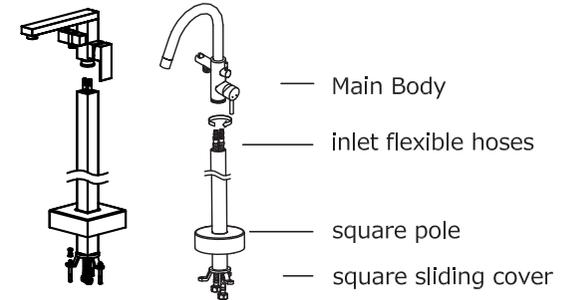
1. Insert the flexible hoses through the square pole and assembling them to main body turning by hand.
