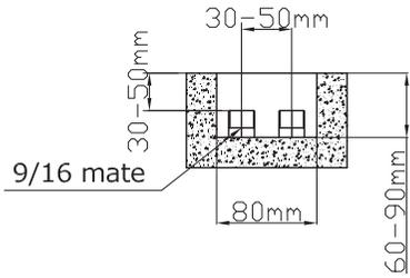
3. Create a chamber in the floor following the above measure with 9/16 male connectors for water net.
