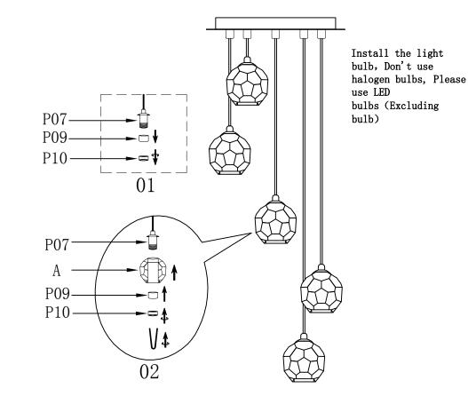
01. Unscrew the lamp holder ring (P10) counterclockwise, and then remove the iron tube (P09);
