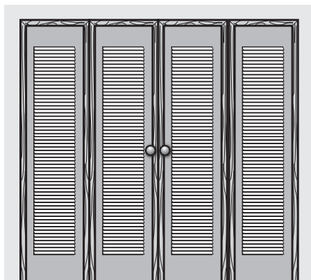
Bi-Fold louvered doors with 120 sq. in of ventilation
