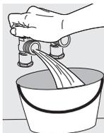
2. Check to ensure that the inlet hoses have the rubber washer firmly in place.
