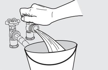
4. Inspect hose couplings for proper placement of rubber washers. Use hoses from ASSEMBLY HOSE KIT# 5304495002 (not included).
