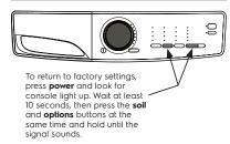
To select or delete an option, press options; then, while the indicator is blinking, press set. The indicator will be illuminated when the option has been selected. The indicator will no longer be lighted when the option has been deleted. See stain option for specific instructions about treating stains with the stain option (on select models).
