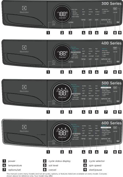
Press the power ① button to turn on the unit Turn the cycle selector ring (on select models) in either direction or repeatedly press the cycles button (on other models) to scroll through the cycles.
