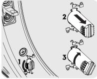
To disengage the stand, rotate to unlock, push the stand in and rotate to lock position.
