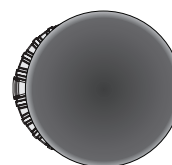
Incorrect Burner Cap Placement
