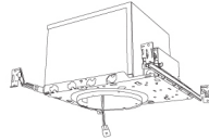
6" ICA Housing New Construction
