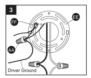
4. Supply wire connection guide: Make wire connections, securing with wire connectors (AA), following the reference chart listed below.
