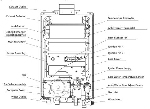
A NOTICE! The Anti-Freezer and its thermostat are for the Indoor water heater, the indoor water heater has the Anti-freeze function only.
