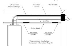
For maintenance and inspection purposes, the following holes are required to be made:
