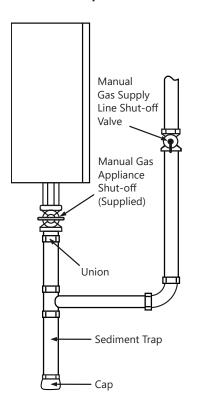
The supplied Manual Gas Appliance Shutoff Valve must be installed at the gas connection of the water heater at the time of installation (see diagram to the left).
