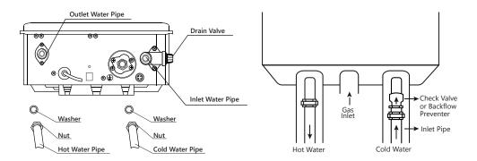
▲NOTICE: The hot and cold pipes should be insulated as shown to help provide additional freeze protection.
