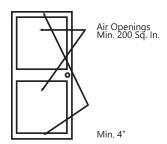
A confined space is one having a volume of less than 50 cubic feet per 1,000 BTUH of the aggregate input of all appliances within that space.
