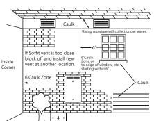
MARNING: Moisture in the flue gas will condense as it leaves the vent terminal. In cold weather this condensate can freeze on the exterior wall, under the eaves and on surrounding objects. Some discoloration to the exterior of the building is to be expected. However, improper location or installation can result in severe damage to the structure or exterior finish of the building. Code requirements are subject to change and may vary by location.
