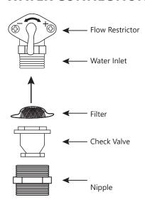
Plumbing should be carried out by a qualified plumber in accordance with local codes. Use approved plumbing materials and tools only.
