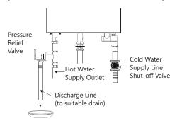
**NOTICE:** Local codes govern the installation of relief valves. If local codes require that a temperature and pressure relief valve should be installed the manufacturer recommends a type 40XL Watts T&P relief valve or an equivalent model be used.
