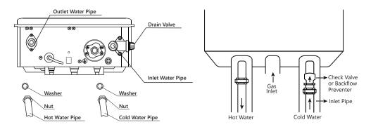
▲NOTICE: The hot and cold pipes should be insulated as shown to help provide additional freeze protection.
