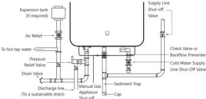
▲ NOTICE: The above illustrates a pressure only relief valve. If local codes require a combination temperature and pressure relief valve be installed, an extension piece may be needed.
