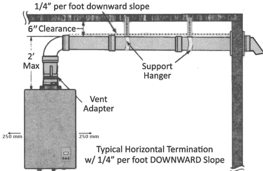
**⚠ WARNING:** Use UL approved Category III vent material only. No other vent material is permitted. Owner must refer to vent manufacturer's instructions and specifications. Z-Flex information can be found at [www.novaflex.com](http://www.novaflex.com), refer to page 32 for additional links.
