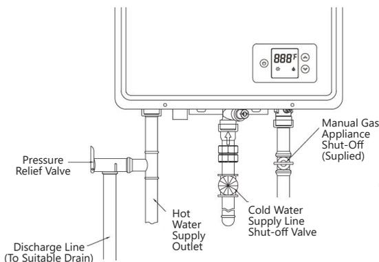
**NOTICE:** Local codes govern the installation of relief valves. If local codes require that a temperature and pressure relief valve should be installed the manufacturer recommends a type 40XL Watts T&P relief valve or an equivalent model be used.
