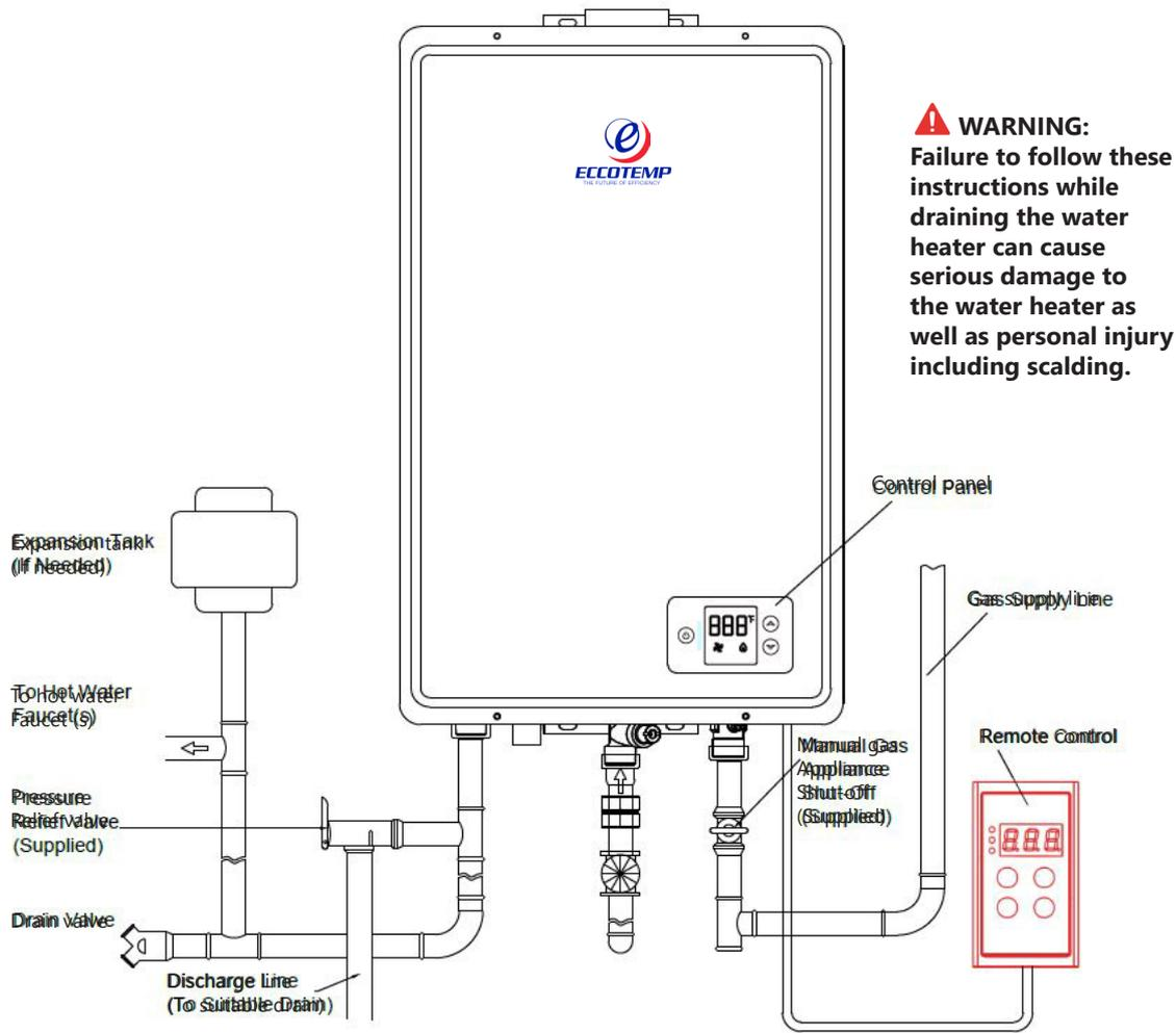
Below are instructions for draining water out of the water heater.
