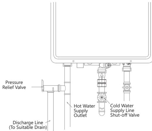
**NOTICE: The above illustrates a pressure only relief valve. If local codes require a combination of temperature and pressure relief, a valve can be installed, but an extension piece may be needed.**
