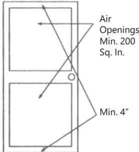
A confined space is one having a volume of less than 50 cubic feet per 1,000 BTUH of the aggregate input of all appliances within that space.
