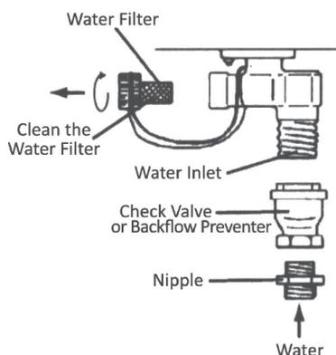
If a water heater is installed in a closed water supply system, such as one having a backflow preventer in the cold water supply line, means shall be provided to control thermal expansion. Contact the water supplier or local plumbing inspector on how to control this situation. Install a shutoff valve near the inlet of the water heater for service and draining purposes.
