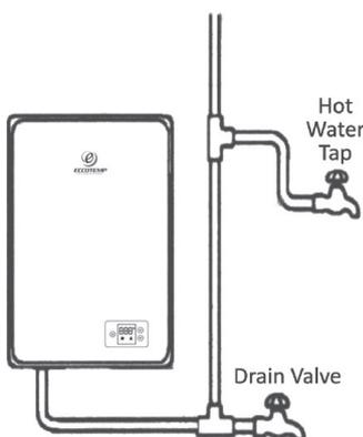
**NOTICE:** The pipes MUST be completely drainable. If the hot water faucets are located at a point higher than the water heater, place a drain valve at the lowest point (see illustration to the bottom left).
