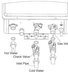
**NOTICE: The hot and cold pipes should be insulated to help provide additional freeze protection.**
