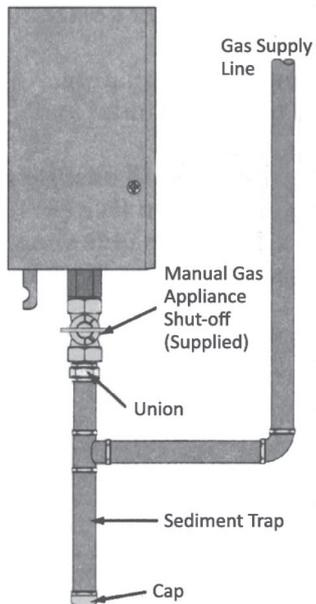
The supplied Manual Gas Appliance Shutoff Valve must be installed at the gas connection of the water heater at the time of installation (see diagram to the left).
