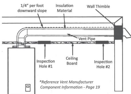
For maintenance and inspection purposes, the following holes are required to be made:
