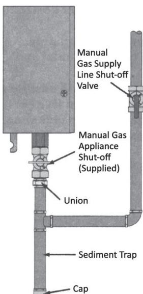
A Manual Gas Appliance Shutoff Valve must be installed at the gas connection of the water heater at the time of installation (see diagram to the left). The branch gas supply line to the water heater should be clean black steel pipe or other approved gas piping material.
