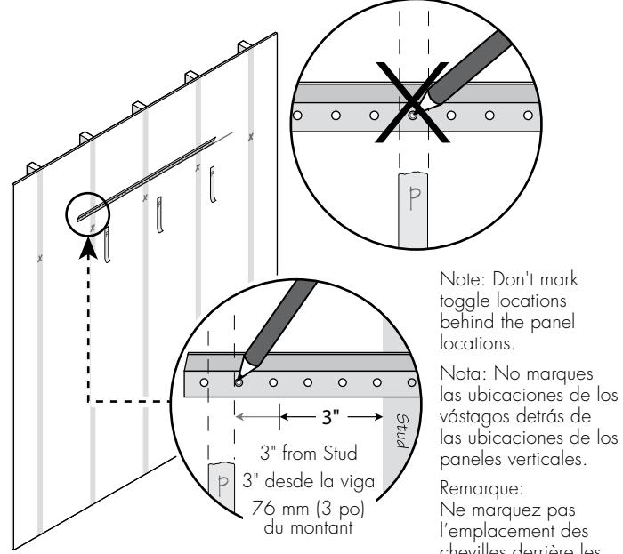
**7** Rotate track out of position, then drill toggle holes. Use  $\frac{1}{2}$ " drill bit.
