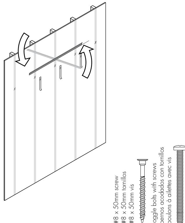
10 To create the tower unit on the floor, attach two shelves to vertical panels using #8 x 50mm screws. If desired, attach screw covers onto screw heads.
