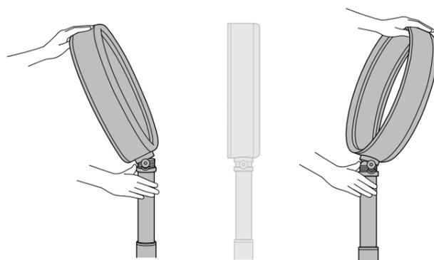
While holding the stand, tilt the loop amplifier towards or away from you to adjust airflow angle.
