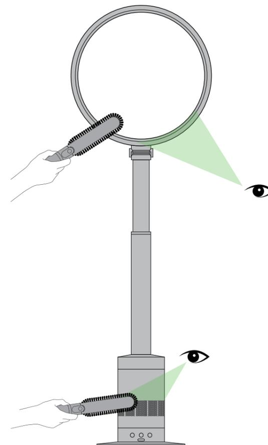
Look for blockages in the air inlet holes and in the small aperture inside the loop amplifier. Use a soft brush to remove debris.
