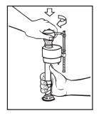
• Replace TOP by engaging lugs and rotating 1/8 turn clockwise. MAKE CERTAIN TIP IS TURNED POSITION. VALVE MAY NOT TURN ON IF TOP IS NOT FULLY TURNED TO THE LOCKED POSITION.
