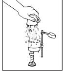
• While holding a container over the uncapped VALVE to prevent splashing, turn water supply on and off TO THE LOCKED a few times. Leave water supply off.
