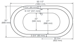
Freestanding tubs use wall-mounted or freestanding faucets. The waste and overflow assembly is concealed between the walls of the tub, eliminating the need for a decorative exposed drain kit.
