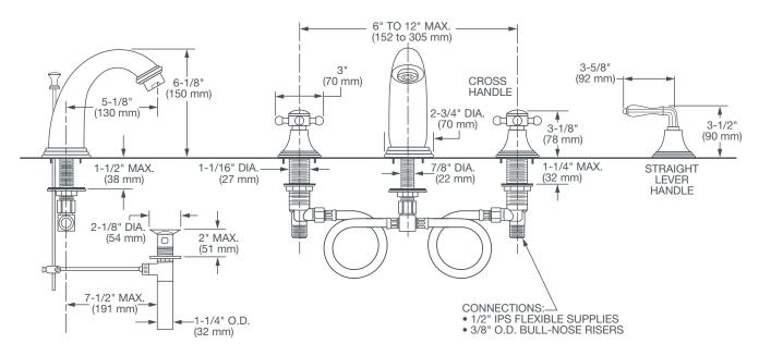
NOTE: MOUNTING HOLES ARE 1-3/8" DIA. (35 mm)
