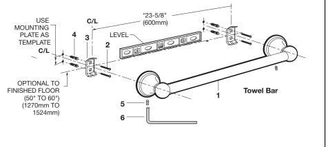
\*FROM CENTER TO CENTER OF WALL BRACKETS \*NOTE: MEASURMENT IS APPROXIMATE ONLY, PLEASE USE BAR AS TEMPLATE FOR ACTUAL CENTER TO CENTER MEASUREMENTS.
