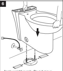
Apply weight evenly. Do not move after placement. Water tight seal may break.
