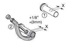
Add dimension Y and 1/8" (3mm). Using that dimension, mark a line on the pipe measuring from the hub side. Cut off the pipe at the line with a pipe cutter.
