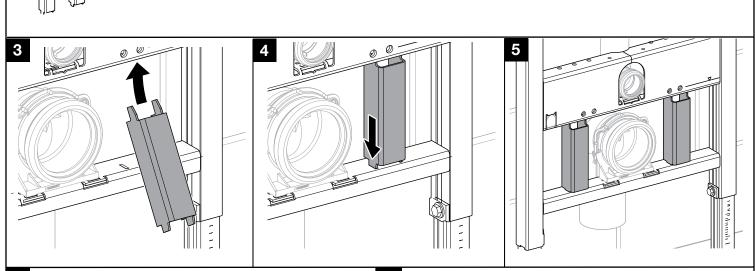
These 2 brackets must be installed during tank frame installation. The brackets are delivered with
