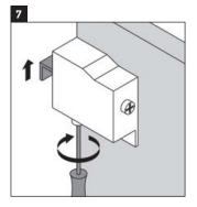
Using a screwdriver, adjust the vanity mounting hinge system clockwise.
