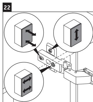
> These screws allow adjustment in three directions: up and down, front to back, and side-to-side. Only if necessary, make minor adjustments to the cabinet front(s), closing the door to check alignment with each adjustment made.
