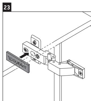
> When adjustment is complete, replace the hinge cover.
