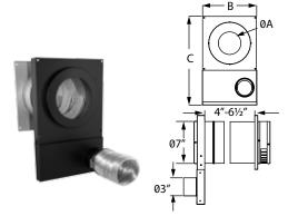
A direct vent for bringing outside air for combustion through an adjustable air channel in wall thimble to appliance without cutting a second hole into the wall. Minimizes down drafts in below-grade installations. Patent-pending.
