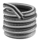
Use when relining masonry chimney for use with biofuel appliances. Made of super-ferritic stainless steel. Must be used with PelletVent Pro Male and Female Flex Adapters. Rigid pipe must be used when terminating system.
