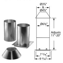
Required for installations that pass through an attic to prevent insulation and debris from accumulating near the vent. Provides 1" clearance to combustibles.
