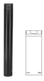
Features fully unitized, twist-lock construction in 3" and 4" diameters. Listed at 1" clearance to combustibles in the USA and Canada. It can be used in both vertical and horizontal installations. Stainless steel welded seam inner wall, combined with a galvalume welded seam outer wall. Pipe OD is diameter plus %". Galvalume or painted black outer finish. 12" length available with stainless steel outer (SS). To calculate installed length, subtract 1 ½" from each length of pipe.
