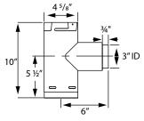
Use for a 90° offset. Attaches directly to appliance as an adapter. Converts a 3" appliance to a 4" PelletVent Pro system. Removable twist-lock Clean-Out Tee Cap.
