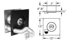
Allows outside fresh air for combustion through the wall thimble without having to cut a second hole into the wall. Comes with an insulation ring to reduce air infiltration where the pipe slips through the thimble. The 2" diameter, 18" length flex hose expands to 5'. Clamps included. Can be used in US and Canada. Patented.
