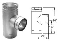
Attaches 3" pipe to branch and 4" pipe to body. Use for a  $90^{\circ}$  offset. Branch swivels for alignment. Removable twist-lock Clean-Out Tee Cap.
