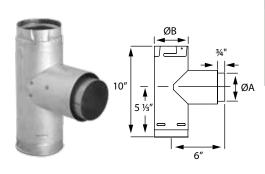
Use for a 90° offset. Attaches directly to appliance as an adapter. Removable twist-lock Clean-Out Tee Cap.
