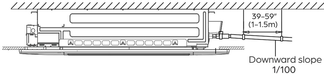
4. This unit is equipped with a drain pump that allows the outlet of the drain pipe to be higher than the pipe's connecting port. The vertical lift pipe must be installed no higher than 29 1/2" (750mm) from the ceiling board. Install hanging wires every 3-5' to keep the drain pipe from sagging, and wrap the indoor portion of the pipe with foam pipe insulation to prevent condensation. Incorrect installation can cause water to flow back into the unit and leaks.
