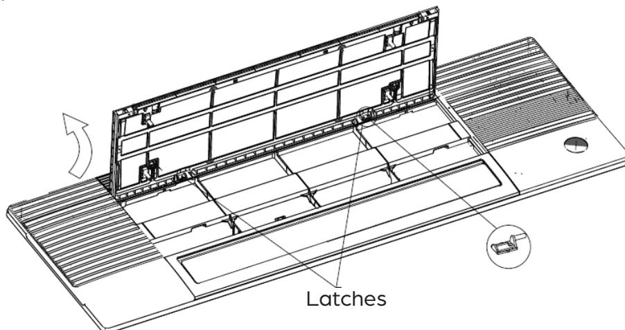
5. Fix the panel to the one-way cassette by two (2) plastic buckles.
