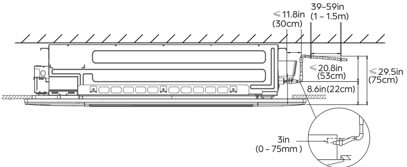
5. If connecting multiple drain pipes, install the pipes as illustrated below.
