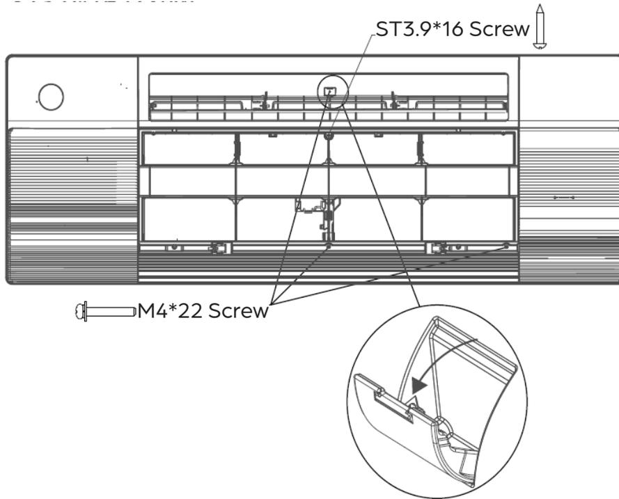
7. Open the two covers on both sides of the panel, fix the panel to the cassette by using 3× M4\*22 screws.
