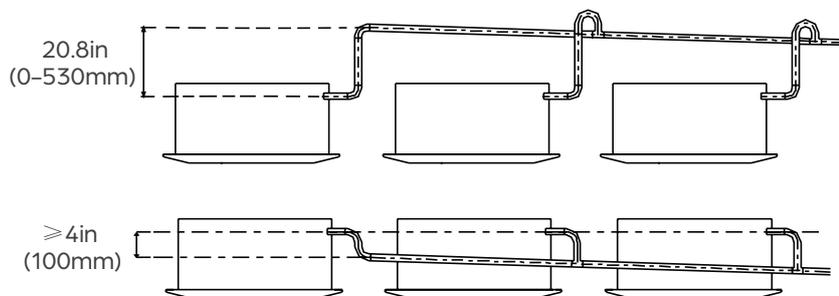
6. Pass the drain pipe through the wall hole to the outside. The end of the pipe should be at least 2" (50mm) above the ground. If it touches the ground, the pipe may become blocked. Make sure the water drains to a safe location where it will not cause water damage or a slipping hazard.
