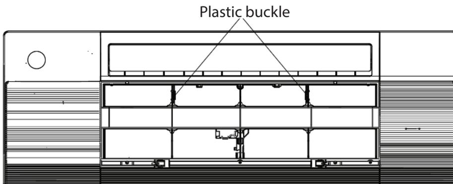
6. Manually rotate the air deflector and fix the panel to the cassette by using 3×M4\*22 screws and a ST3.9\*16 screw.
