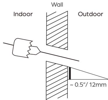
3. Place the protective wall hole sleeve (field supplied) into the hole. This protects pipes and cables from sharp edges and will help seal the opening when you finish the installation process. After the sleeve is inserted through the wall, connect the wall hole sleeve cover to the wall sleeve on the outside end. Make sure the cover is flush with the outside wall.
