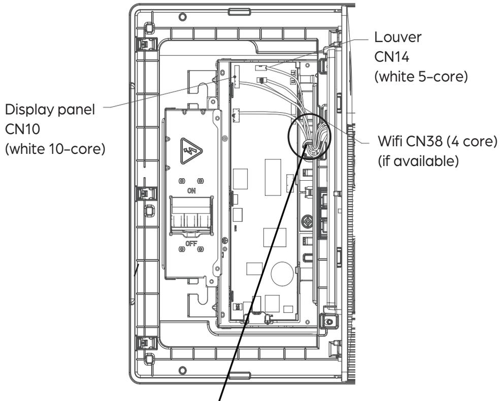
When the connection is completed, please clip the wires to the buckle.
