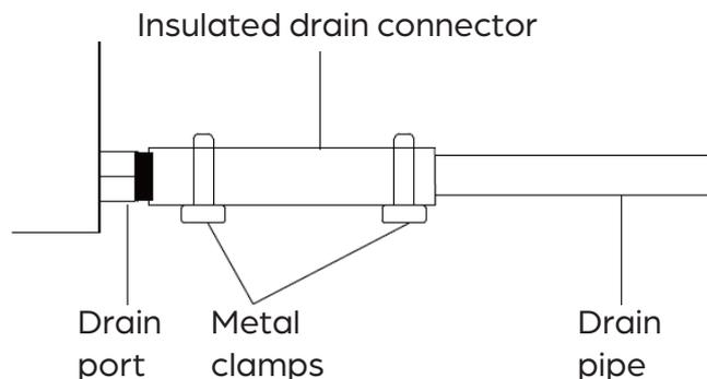
2. Insulate the connecting port and pipe with the accessory sheath (sleeve) provided.
