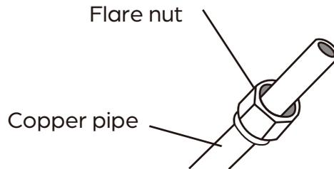
4. Remove PVC tape from ends of pipe when ready to perform flaring.
