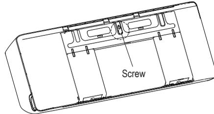
2. Secure the mounting plate to the wall with the anchors and screws provided. Make sure that mounting plate is flat against the wall, and is level.
