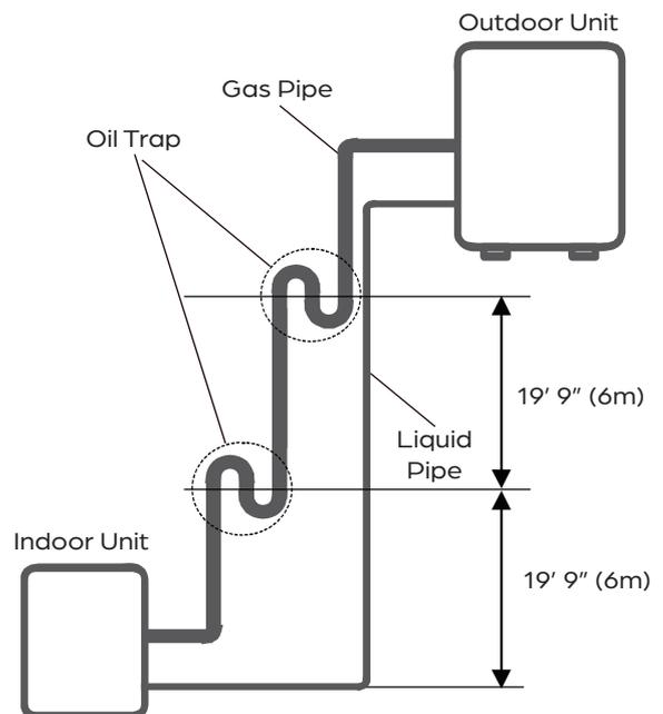
Required distance between oil traps when the outdoor unit is installed higher than the indoor unit.
