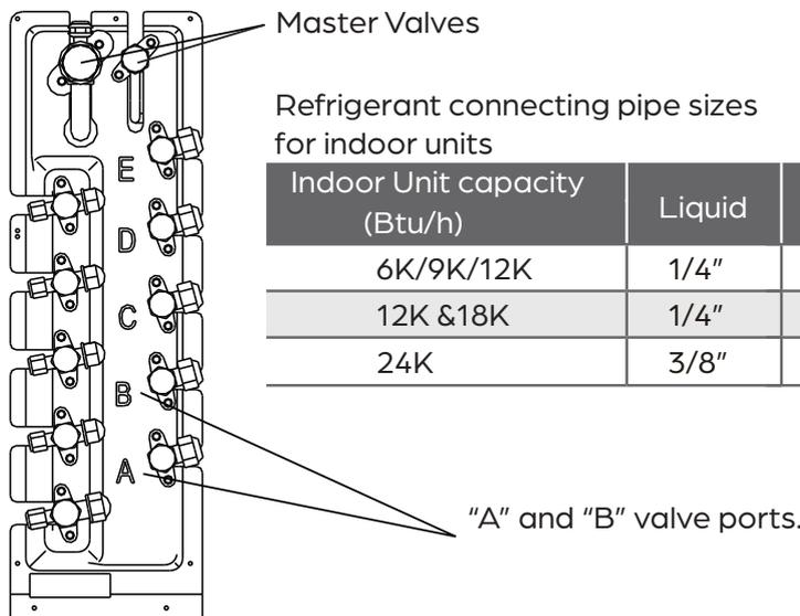
Refrigerant connecting pipe sizes for indoor units
