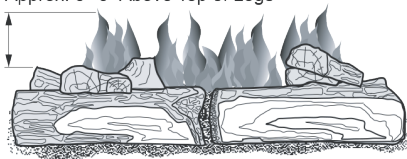
Figure 19 - Correct Burner Flame Pattern
