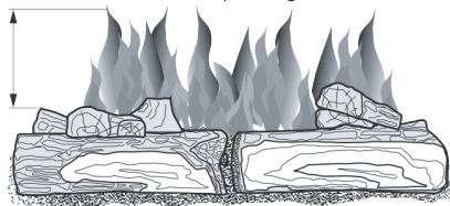
Figure 20 - Incorrect Burner Flame Pattern
