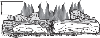
Figure 32 - Correct Burner Flame Pattern with Control Knob Set to HI (5)
