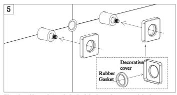
Place the rubber gasket on the back of the decorative cover and slowly pass through the body switch to the wall.
