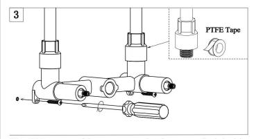
Wrap PTFE tape around the connector, screw into the corresponding hole of the faucet body. Fix the concealed body in the hole slot, (Note: Please ensure the parallelism and perpendicularity of the faucet body before tightening the screws.) Then fill the hole slots.
