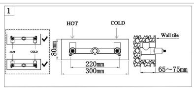
The size of the pre-slotting in the wall: Length:300mm,width:100mm,depth:68~78mm after wall decoration. (Note: Please confirm the thickness of wall decoration before grooving).
