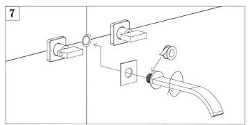
Wrap the PTFE tape around the connector of the spout, and insert the decorative sheet and spout throw into the corresponding hole in turn to complete the installation.
