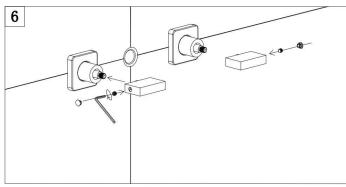
Install the hand wheel into the body switch, tighten the screw with the allen key, then Install the button.
