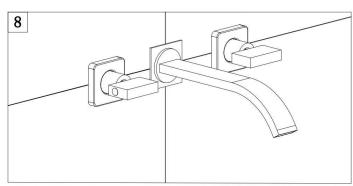
After installation, please ensure that the left for the hot water, and the right for the cold water.
