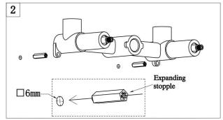
Mark pre-assembly holes on the wall, drill holes with a 6mm drill bit, and then drive Expanding stopple into the holes.
