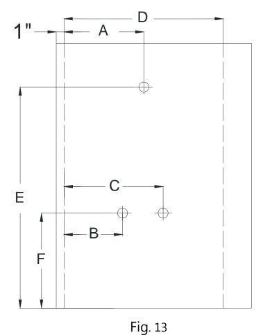
11. Determine which **Side panel (01)** will be installed on the side wall with the fixture.
