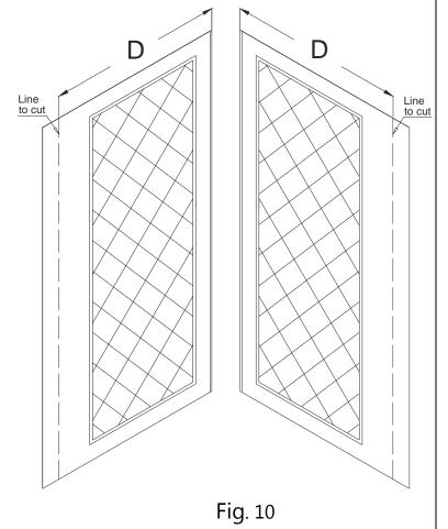
9. Place the **Side panel (01)** on a flat piece of plywood or particle board. Use a sharp industrial knife and a T-square to score along the marked wide ends of the **Side panel** and continue scoring until you have fully cut through the panel.
