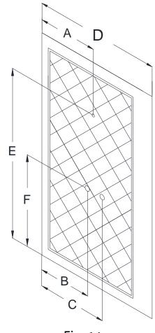
12. Drill the holes for the fixtures in the **Side panel (01)** using the proper diameter saw bit or a handheld jig saw.
