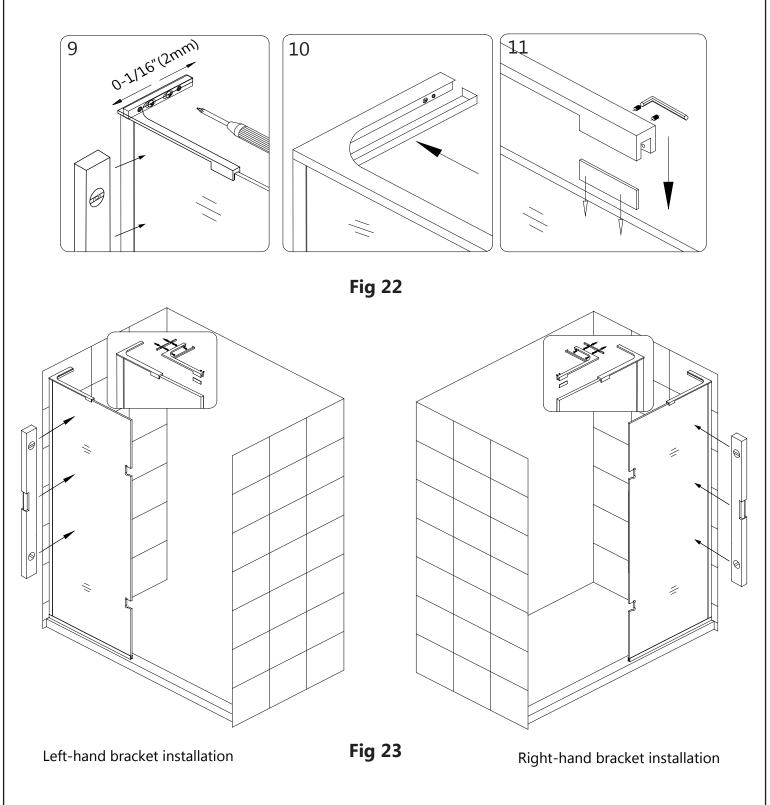
NOTE: The left-hand L-bracket installation is shown. Follow the same steps for installing the right-hand L-bracket.
