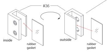
NOTE: The Hinge Panel Glass Bracket (#36) is only to be installed with the 6" Hinge Panel Glass (#32) for the UNIDOOR-X models.
