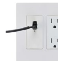
Plug the Safety Interlock Connector into the Interlock Switch Connector.
