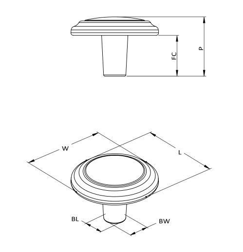
L (Length)=1 1/4"[1.25in] W (Width)=1 1/4"[1.25in] P (Projection)=7/8"[0.875in] FC (Finger Clearance)=9/16"[0.5625in] BL (Base Length)=5/16"[0.3125in] BW (Base Width)=5/16"[0.3125in]
