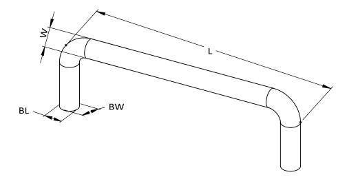
C2C (Center-to-Center)=96 MM[3.779in] L (Length)=4 1/16"[4.0625in] W (Width)=5/16"[0.3125in] P (Projection)=1 1/4"[1.25in] FC (Finger Clearance)=15/16"[0.9375in] BL (Base Length)=5/16"[0.3125in] BW (Base Width)=5/16"[0.3125in]
