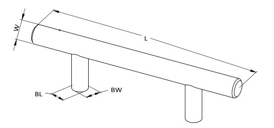
C2C (Center-to-Center)=3"[3.0in] L (Length)=5 3/8"[5.375in] W (Width)=1/2"[0.5in] P (Projection)=1 3/8"[1.375in] FC (Finger Clearance)=7/8"[0.875in] BL (Base Length)=3/8"[0.375in] BW (Base Width)=3/8"[0.375in]
