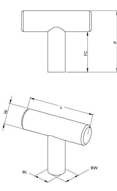
L (Length)=1 9/16"[1.5625in] W (Width)=1/2"[0.5in] P (Projection)=1 3/8"[1.375in] FC (Finger Clearance)=7/8"[0.875in] BL (Base Length)=3/8"[0.375in] BW (Base Width)=3/8"[0.375in]
