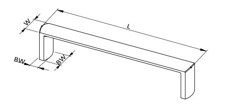
C2C (Center-to-Center)=128 MM[5.039in] L (Length)=5 5/16"[5.354in] W (Width)=5/8"[0.625in] P (Projection)=1 1/16"[1.0625in] FC (Finger Clearance)=7/8"[0.875in] BL (Base Length)=5/16"[0.3125in] BW (Base Width)=5/8"[0.625in]
