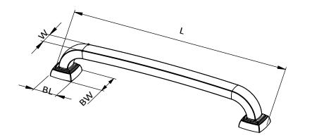
C2C (Center-to-Center)=160 MM[6.299in] L (Length)=7 1/16"[7.0625in] W (Width)=7/16"[0.4375in] P (Projection)=1 3/16"[1.1875in] FC (Finger Clearance)=13/16"[0.8125in] BL (Base Length)=3/4"[0.75in] BW (Base Width)=3/4"[0.75in]
