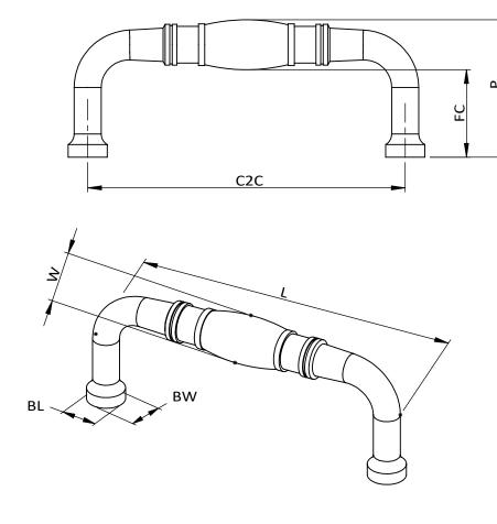
C2C (Center-to-Center)=3"[3.0in] L (Length)=3 3/8"[3.375in] W (Width)=1/2"[0.5in] P (Projection)=1 3/8"[1.375in] FC (Finger Clearance)=7/8"[0.875in] BL (Base Length)=3/8"[0.375in] BW (Base Width)=3/8"[0.375in]
