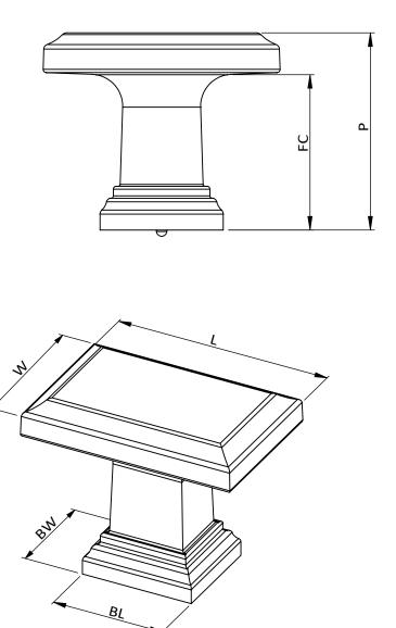
L (Length)=1 1/2"[1.50in] W (Width)=1"[1.0in] P (Projection)=1 1/4"[1.25in] FC (Finger Clearance)=1"[1.0in] BL (Base Length)=13/16"[0.8125in] BW (Base Width)=11/16"[0.6875in]
