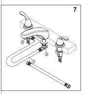
Connect the flexible water supply hose (1) to the bottom of valve bodies (2) as show. Align T-tube (3) in a position which will allow maximum clearance to connect hoses.
