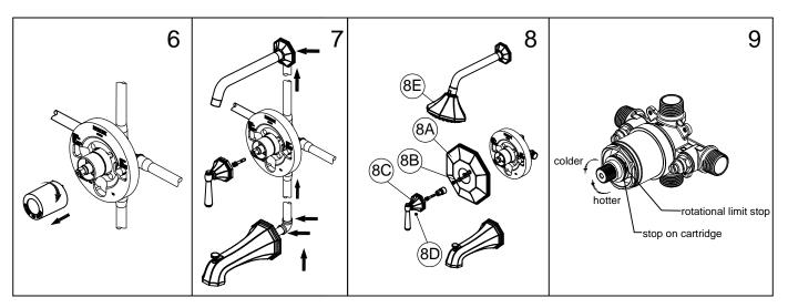
6.Before installing escutcheon, remove the plastic cap from plaster guard by twisting cap in a clockwise direction. Remove the screw from the inverter.
